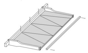
Nail the wedge onto the top bar, trapping the bent wires. Nail through each loop of wire at a slight angle. Fit and nail the second bottom bar.
