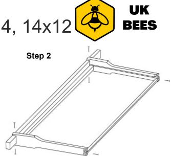
Nail as shown – 2 nails for each side bar, and nail bottom bar up through side bar when nailing Hoffman frames.
