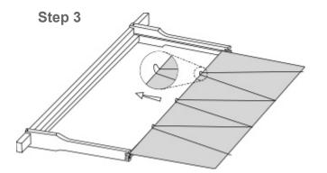
Bend over long wire loops of foundation. Slide foundation along grooves onto top bar.
