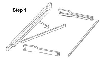
Remove the wedge from the top bar. Assemble the top bar, side bars and one bottom bar. Side bars have the groove on the inside.
